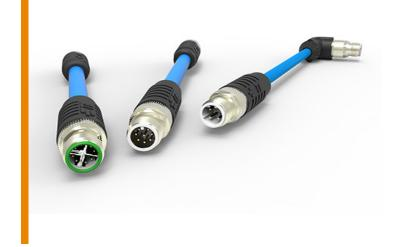
TE Connectivity's M12 cable assemblies fit heavy industrial applications. The cables are pre-assembled so customers can reduce installation time. With its ruggedized design and contacts, the cable can withstand severe shocks and vibrations according to EN 61373 Cat1 Class B.
