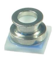
Expanding the digital pressure sensor module family, TE Connectivity (TE) introduces the high linearity and low power MS5837-30BA waterproof digital pressure sensor. Capable of a water depth resolution of 2mm, this factory calibrated, absolute sensor offers different operation modes that allow the user to optimize for conversion speed and power consumption. The water resistant MS5837-30BA can be interfaced to virtually any microcontroller.
